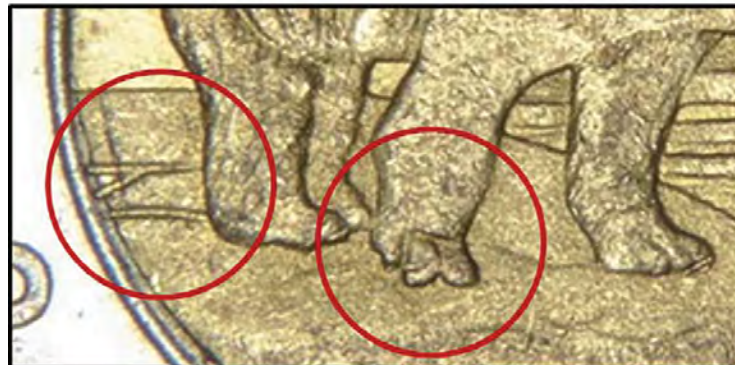
Counterfeit $2 circulation coins (bottom) feature a flaw on the obverse polar bear's front right paw plus less definition in the background design. A genuine toonie is shown at the top.
